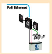
On-board RS-485 channel makes it easy to provide connectivity to other RBH and 3rd party devices, such as: readers, burglar alarm panels, automation systems, etc.
